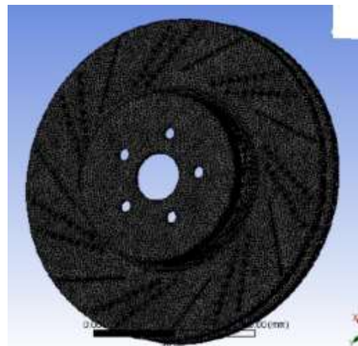
Figure- 2: Meshing of Disc Rotor
