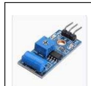
Fig-1: Vibration Sensor
