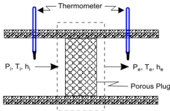
A gas at pressure and temperature flows continuously through a porous plug in a tube and emerges into a space which is maintained at a constant pressure  $P_e$ . The device is thermally insulated and kept horizontal. Consider the dotted portion as control volume.
