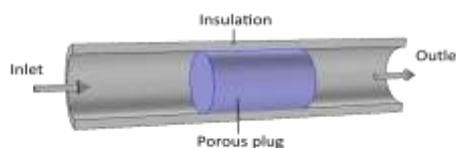
The temperature change pertaining to the Joule-Thomson effect can occur when a flowing gas passes through a pressure regulator, which acts as a throttling device, valve, or porous plug. Here, a temperature change is not necessarily desirable. To balance out any Joule-Thomson related temperature changes, a heating or cooling element can be used.
