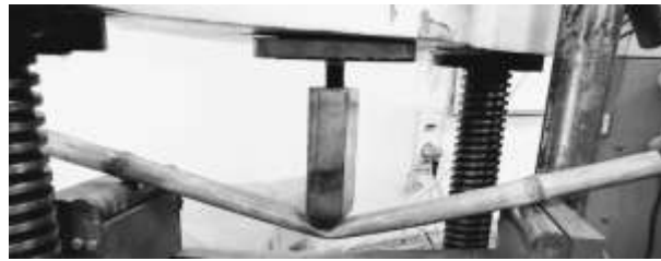
Fig.3 Flexure test of bamboo
