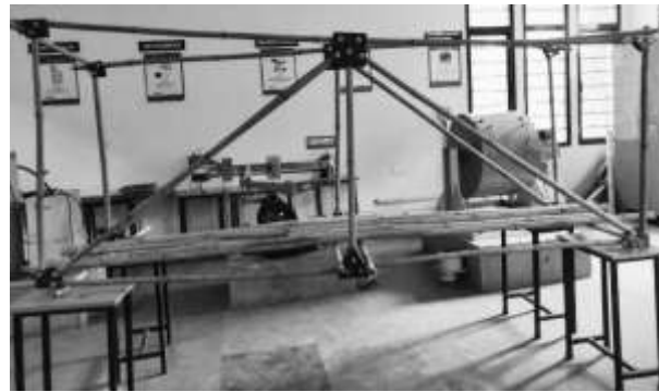
Fig. 9 fabricated bamboo truss
