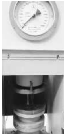
Fig.2 Compression test of bamboo
