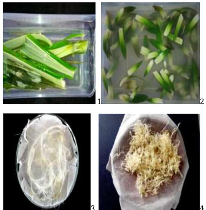
Figure: 1.Agava cantala leaves, 2. pineapple leaves, 3 Extracted Agava cantala fibers, 4.Extracted Pineapple fibers
