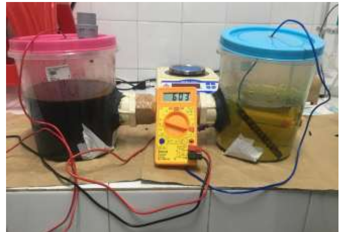
Fig -1: Experimental Setup of MFC during inoculation period
