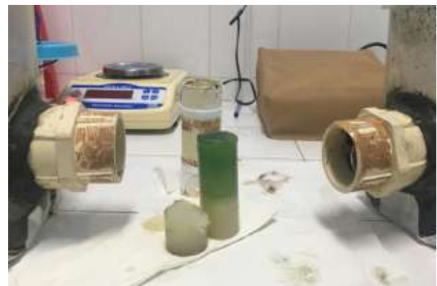
Fig -2: Exhausted Salt Bridge
