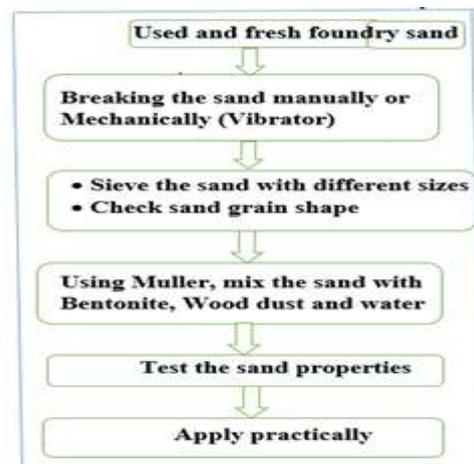
**Fig. 4:** Conceptual framework of recycled sand preparation
