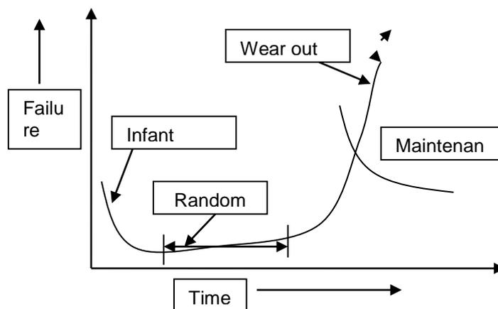
The cycle starts with a high probability of premature (infant) failures that result from manufacturing or installation errors. The curves shown failure probability verses time required. In this failure cycle shows the various type of failure and time required for repair it. The probability of failures is then relatively level until the equipment begins to wear out. Preventive maintenance is scheduled to take place before this probability increases significantly.
