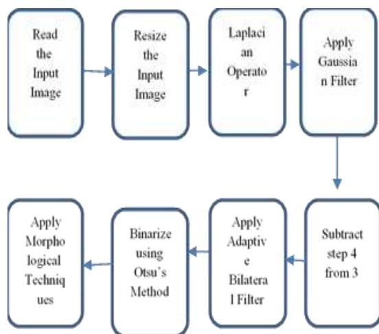
Fig- 4: Block diagram
