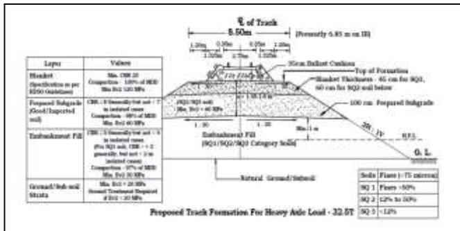
Fig -1: Proposed Track Formation for RDSO Heavy Axle Load - 32.5T
