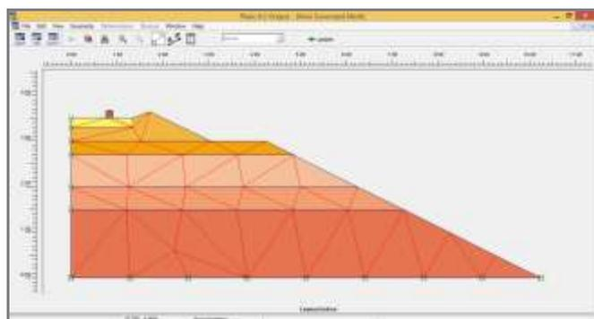
Fig -2: Geometry of Railway Ballast Embankment
