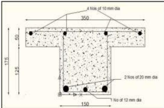
Fig -1: Reinforcement Detailing of T- Beam
