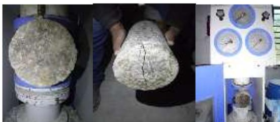
Fig .4 Split tensile testing specimens
