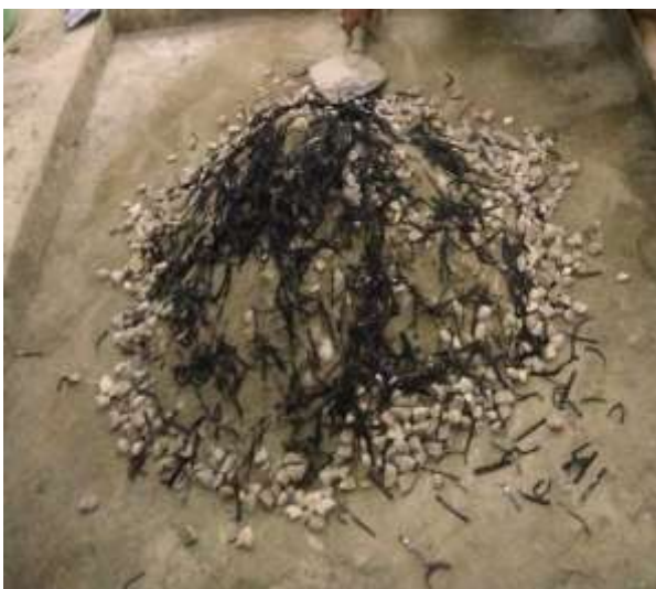
Figure 8 Preparation of concrete mix with Bagasse Ash coated PET fiber
