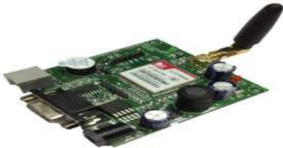
**Fig -4 GSM Module**
