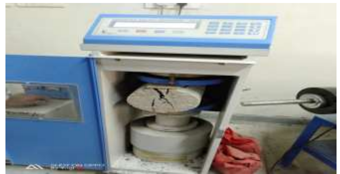
Fig -2: Failure of Specimen
