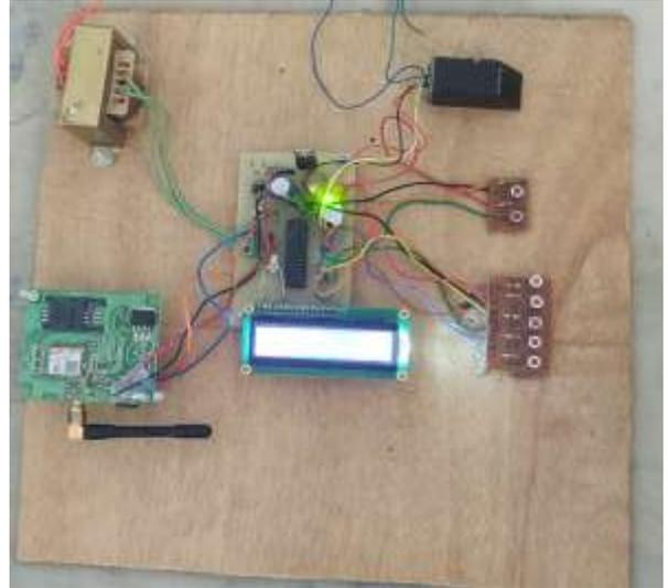
Figure 2 biometric EVM using Arduino Software
