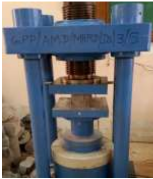
Fig- 2: Universal testing machine to determine the compressive strength of bricks specimen
