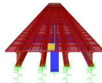
**Fig -1:** Front view model of conventional prestressed bridge superstructure
