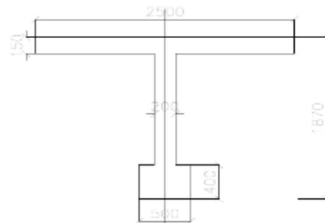
Fig -4: Cross section of main girder
