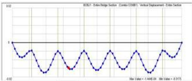
Fig -13: Bridge response plot for maximum displacement
