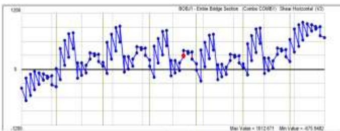
Fig -11: Bridge response plot for maximum shear value
