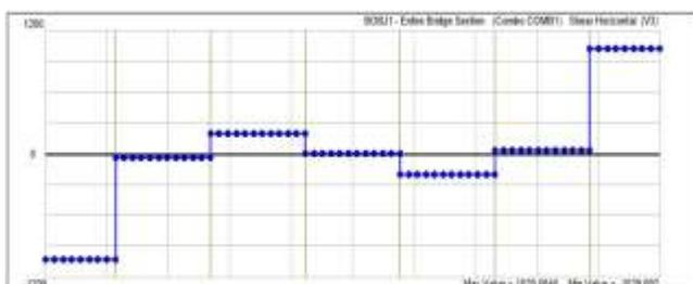
Fig- 5: Bridge response plot for maximum shear value
