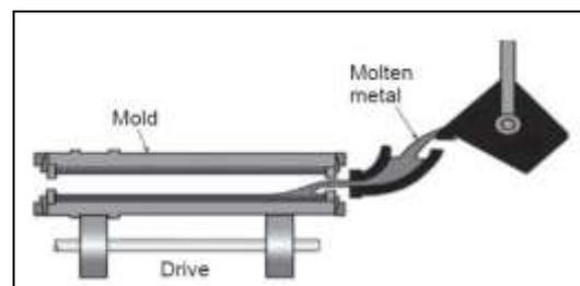
Fig -1: Schematic of horizontal centrifugal casting[2]
