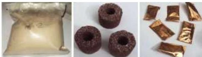
**Fig -2:** Albral 2 flux, Degassing Tablet & Deoxidising tubes
