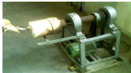
Fig -2: Horizontal centrifugal casting machine setup
