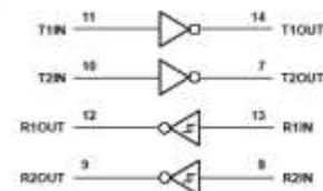
In this circuit the microcontroller transmitter pin is connected in the MAX232 T2IN pin which converts input 5v TTL/CMOS level to RS232 level. Then T2OUT pin is connected to receiver pin of 9 pin D type serial connector which is directly connected to PC.
