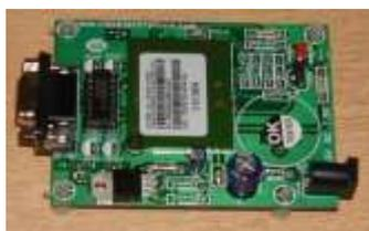
This GSM Modem can accept any GSM network operator SIM card and act just like a mobile phone with its own unique phone number.
