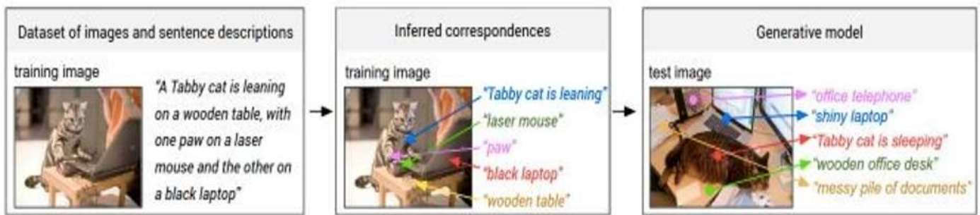
Fig 1. A dataset of images and their sentence descriptions is given as input and the model infers correspondences and learns to generate novel descriptions.
