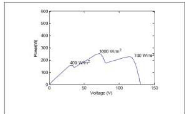
Fig 4: Power Vs. Voltage Curve of PV Array under partial shading condition
