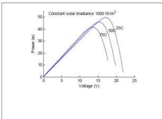
Fig 3: Power Vs. Voltage Curve of PV panel for Variable Temperatures
