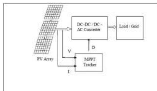
Fig. 1 Solar PV system with MPPT
