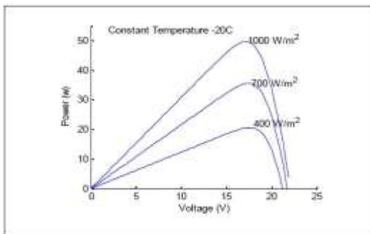
Fig.2 Power vs. Voltage Curve of PV panel for Variable Irradiances
