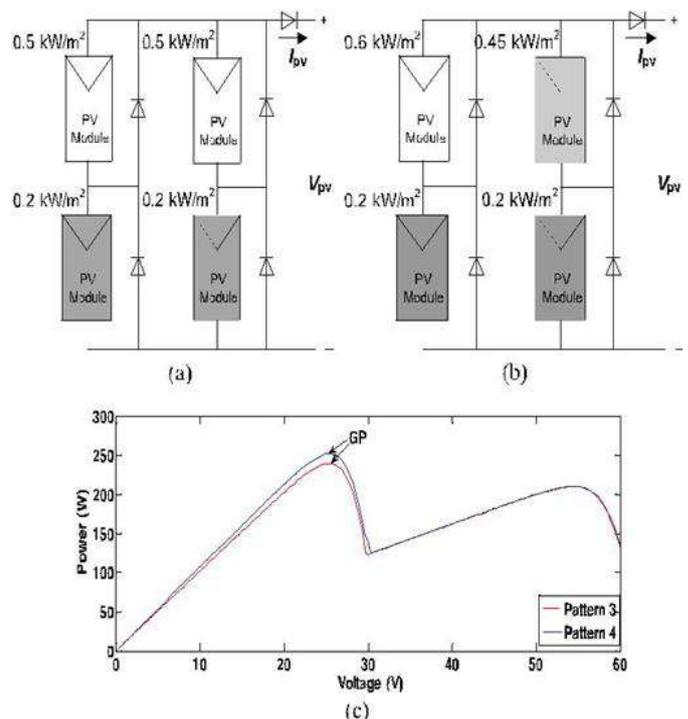
Fig.6. 2S2P configuration under different shading patterns. (a) Pattern 3.(b) Pattern 4. (c) P -V curves under PSCs.
