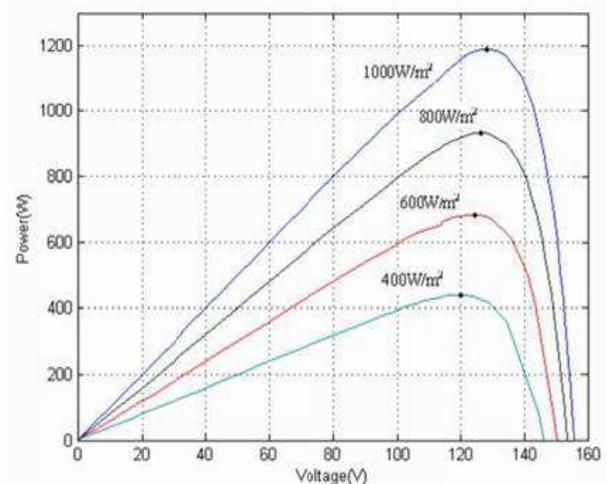
Fig.7.Pv curve of solar array for different irradiation and constant temperature of 25°C
