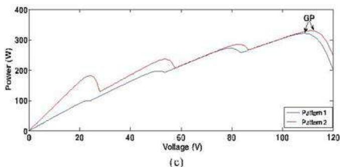
Fig. 5. 4S Configuration under different shading patterns. (a) Pattern 1. (b) Pattern 2. (c) P-V curves under PSCs.
