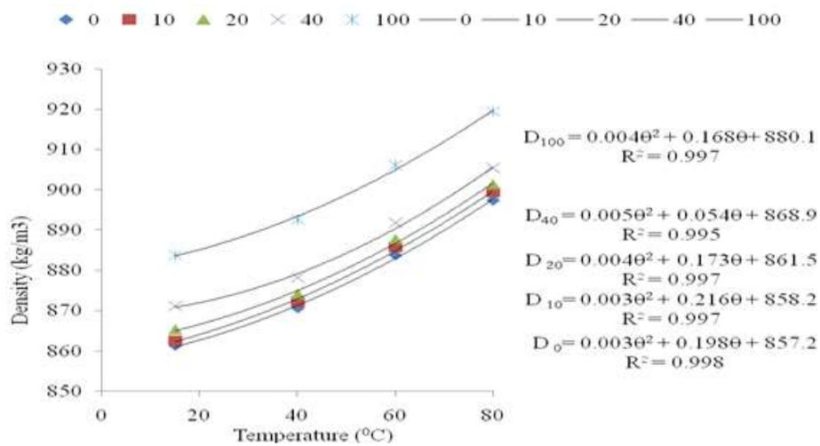
Figure 3 Variation of density of fuel types with temperature
