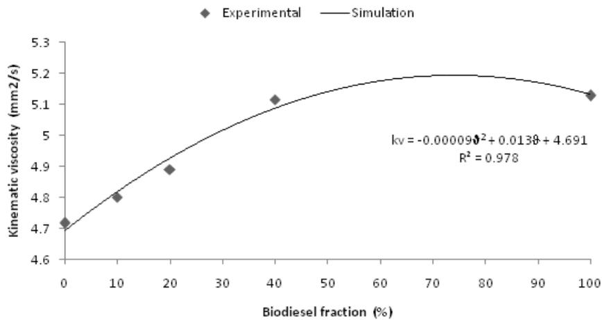
Figure 2 Variation of kinematic viscosity with biodiesel fraction
