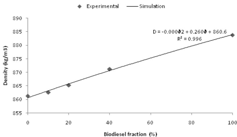
**Figure 1** Variation of density with biodiesel fraction
