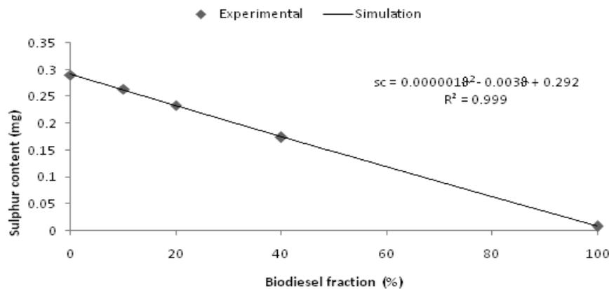
Figure 6 Variation of sulphur content with biodiesel fraction
