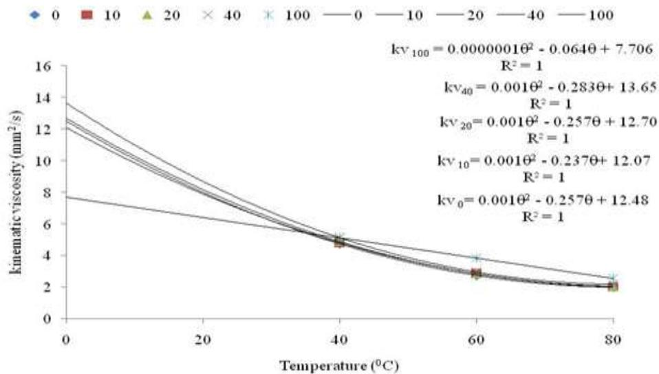
Figure 4 Variation of kinematic viscosity of fuel types with temperature
