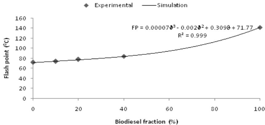
Figure 5 Variation of flash point with biodiesel fraction
