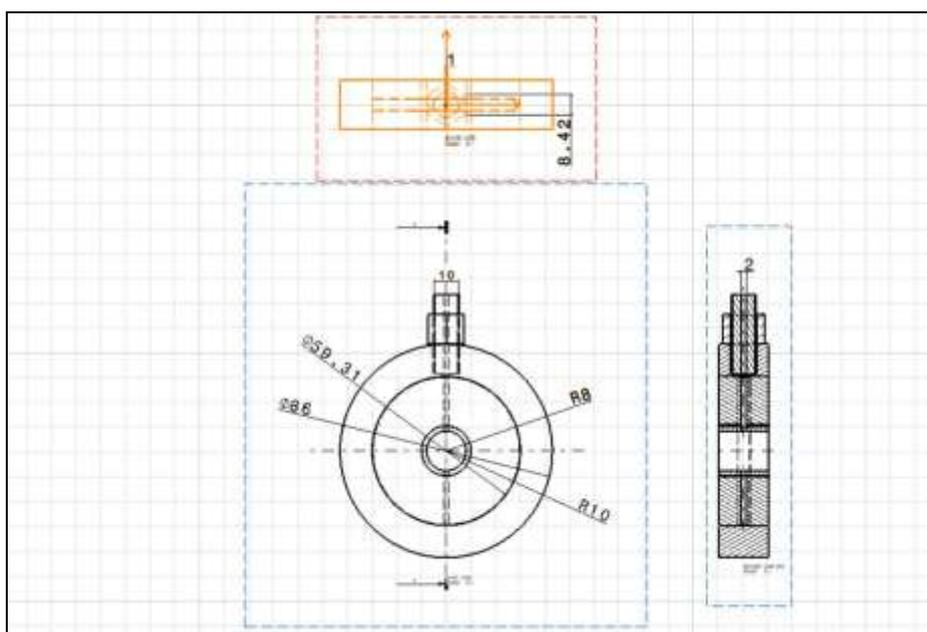
**Fig 3.1.1** Drafting of air ring gauge
