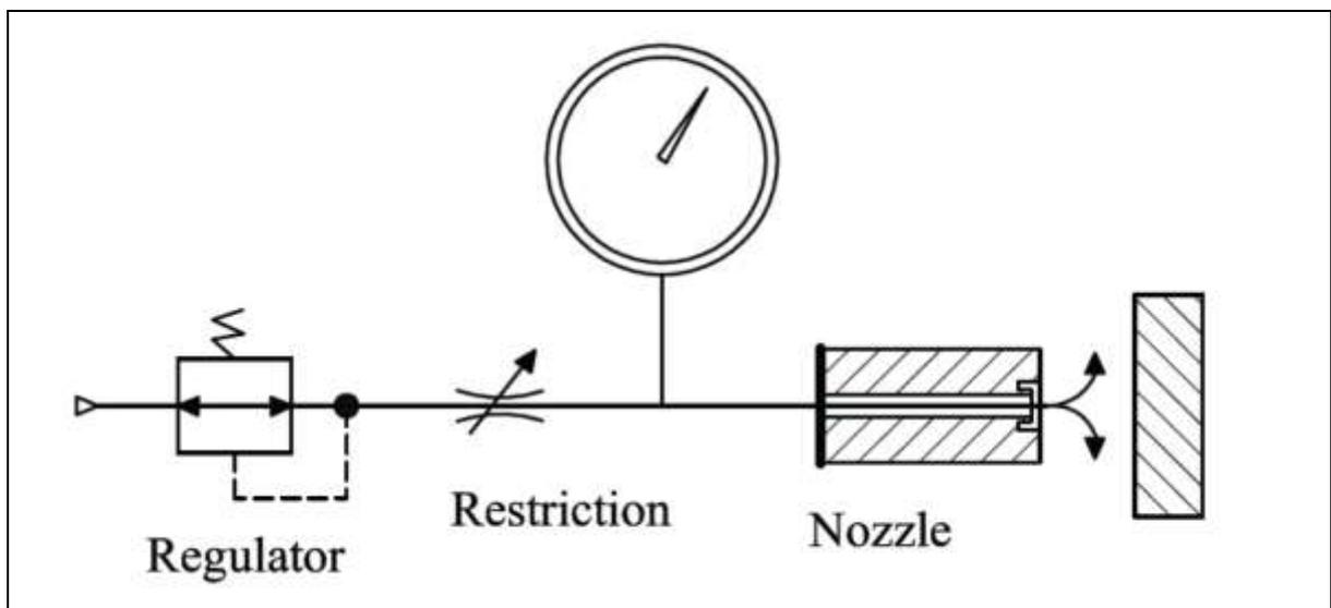
Fig.1.2.1 Simple air circuit.
