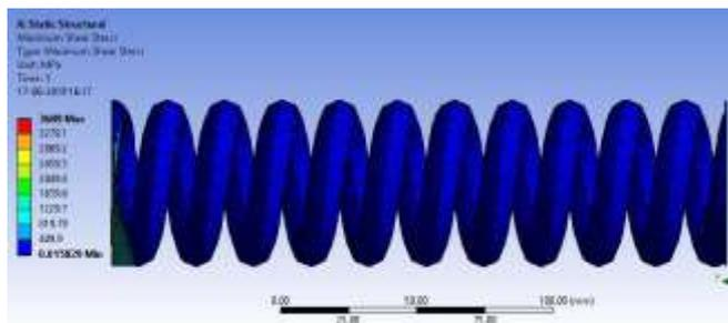
Fig 7: Max Shear stress in hollow circular profile spring
