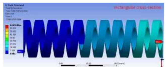
Fig 3: Deformation in hollow rectangular profile spring
