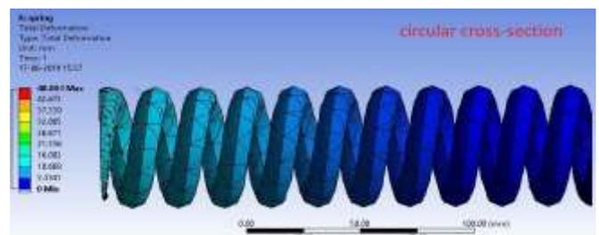
Fig 1: Deformation in circular profile spring in mm
