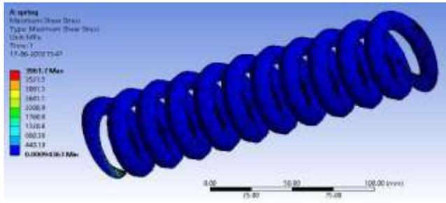
Fig 6: Max Shear stress in circular profile spring
