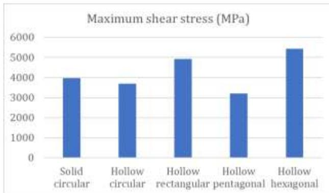
Fig 12: Graph showing shear stress of various profiles under static structural analysis
