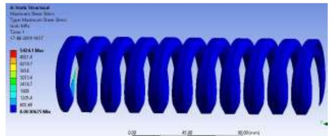
Fig 10: Max Shear stress in hollow hexagonal profile spring
