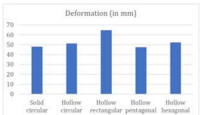
Fig 11: Graph showing deformation of various profiles under static structural analysis
