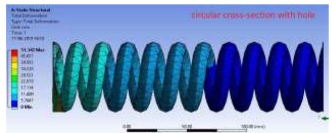
Fig 2: Deformation in hollow circular profile spring
