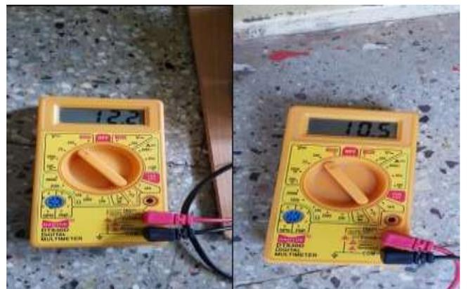
**Fig.4** Output voltage of charge controller and Solar panel
