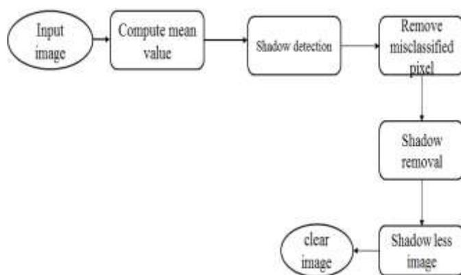
Figure 2: Shadow removal system architecture
