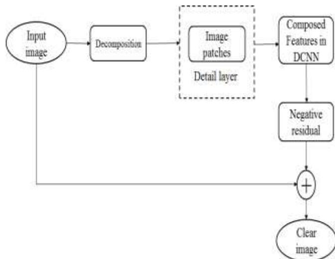
Figure 1: Rain streaks removal system architecture
