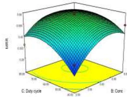
Fig. 3.6 Variation of MRR with Duty cycle and Concentration
