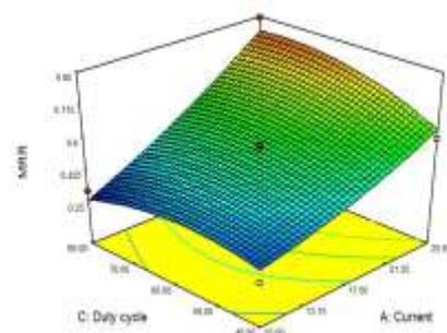
Fig 3.7 Variation of MRR with Duty cycle and Current
