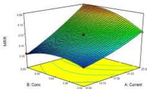
Fig.3.5 Variation of MRR with Current and Concentration
