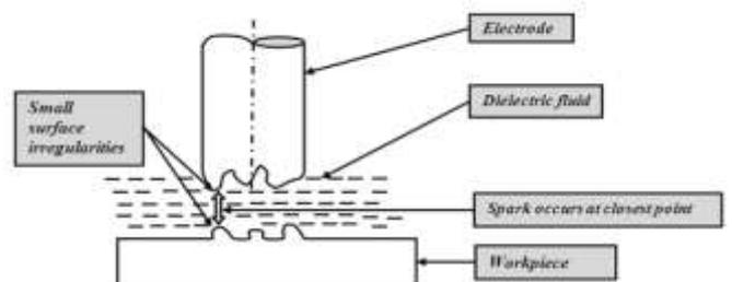
Fig 2.4 Working principle of EDM
