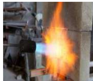
Figure 1 precast concrete fire resistance
