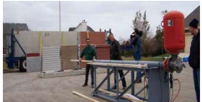
Figure 3 testing of wall against tornado
