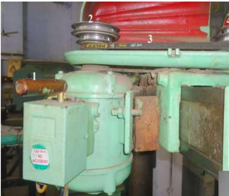
**Figure 2.1 Arrangement for changing the drill speed**
