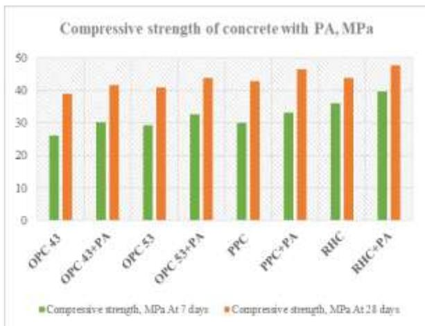
Figure 1.4 shows the graph of combinations of concrete with PA versus compressive strength, MPa
