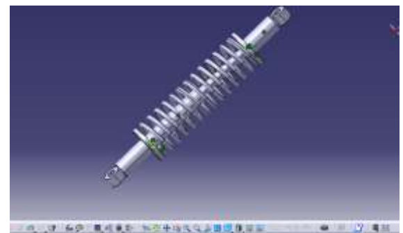
Fig: 3.3.5 Assembly of shock absorber
