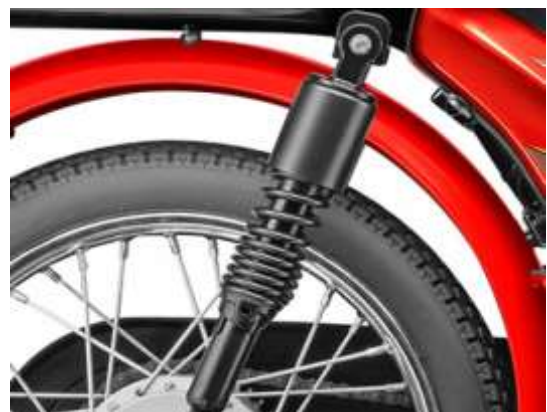
Fig: 1.3.1 Rear shock absorber and spring
