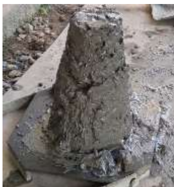
Fig-3: Slump cone test
