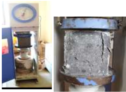
Fig-4: Compressive strength testing of specimen
