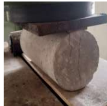
Fig-6: Split tensile strength testing of specimen
