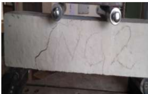
Fig-7: Flexural strength testing of specimen
