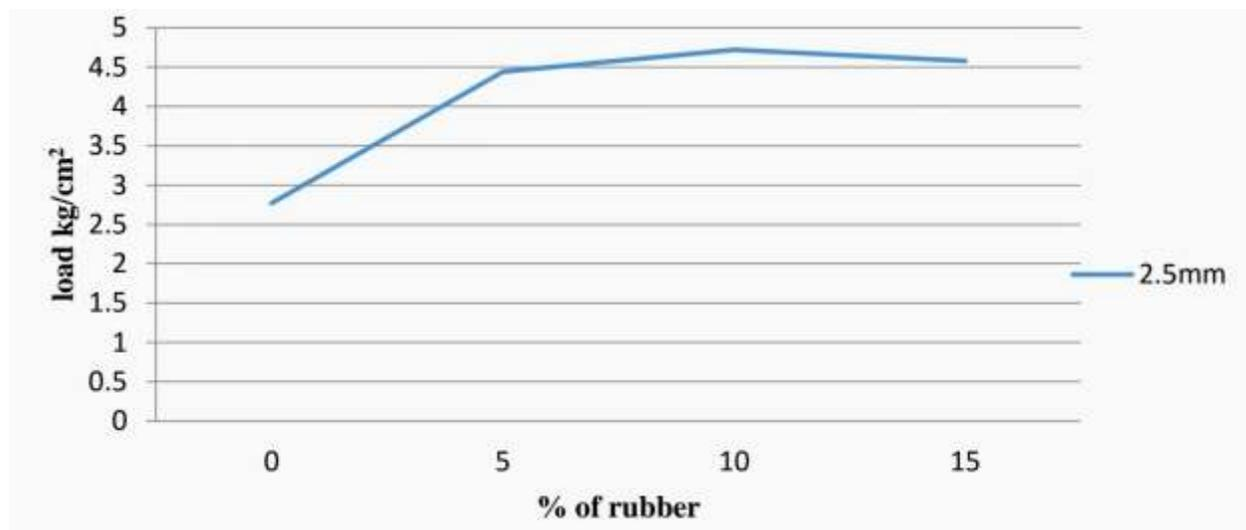
Figure:3 Graph of direct shear for black cotton soil
