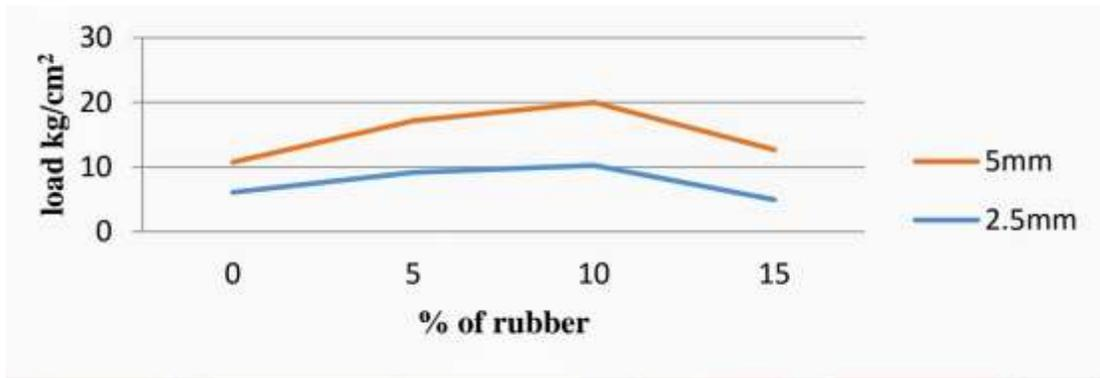
Figure: 2 Graph of California bearing ratio for black cotton soil
