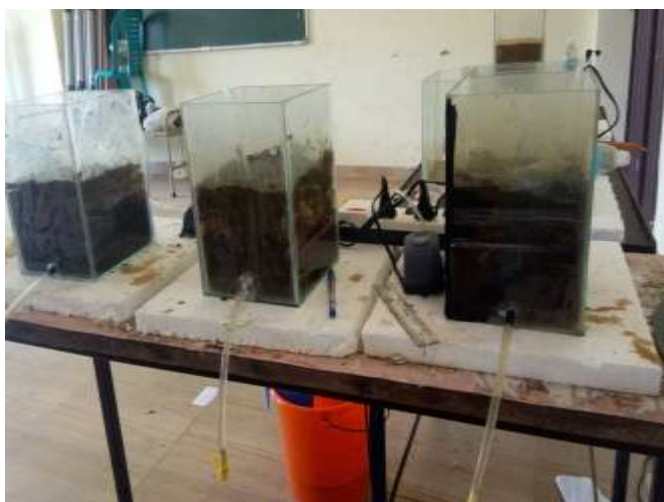
Fig-1: Reactor Seeded with Cowdung
