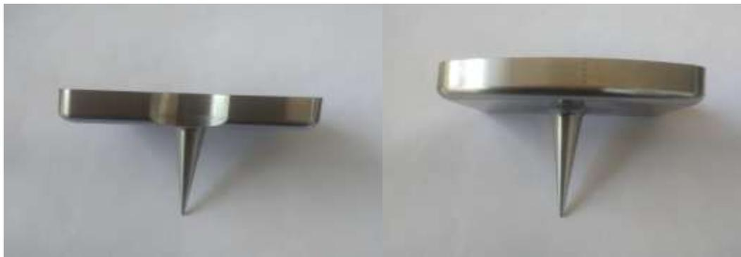
Fig. 4 Fabricated tibial component
