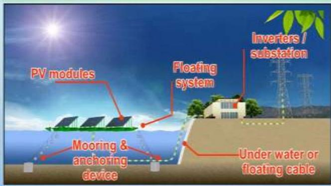
Fig -1: Schematic of FPV system
