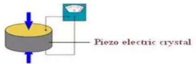
Fig.1.2 Generation of ultrasound using piezoelectric method
