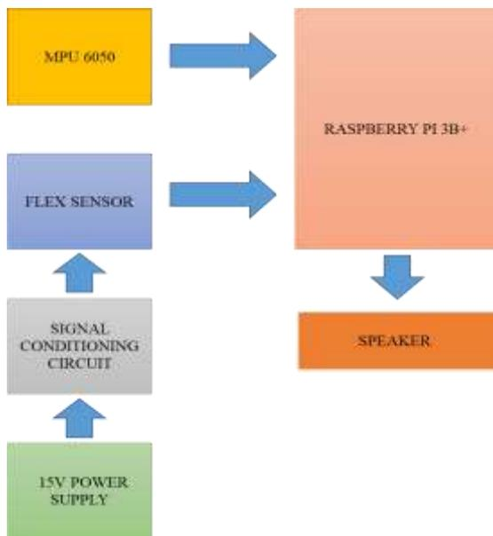
Fig- 2: System block diagram
