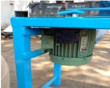
Figure 5.2 d: Connection of motor shaft to shake table frame
