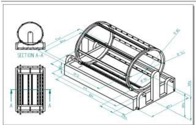
Fig. 5.2.2 sectional front view, top view & isometric view
