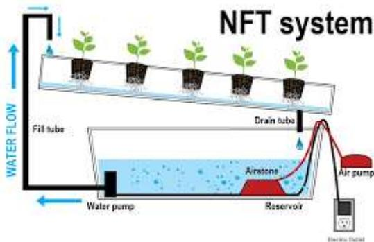
Fig. 4.1.1 Above figure shows overall view about the hydroponics NFT system.
