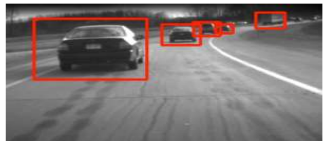
Fig-5: Indicates the vehicle detection
