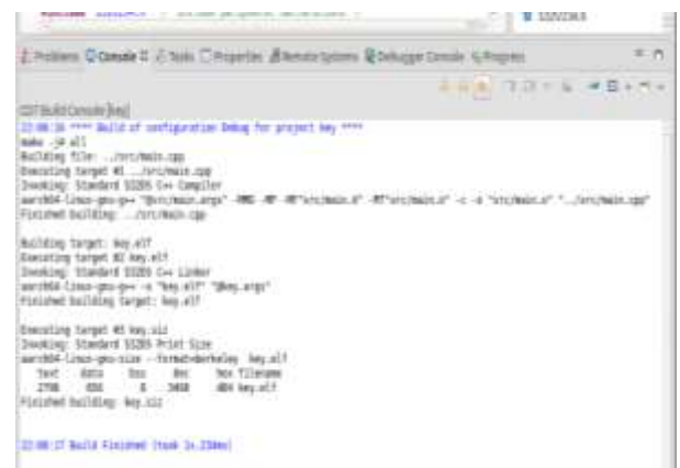
Fig-6:Indicates the building of code and genertion of .elf file
