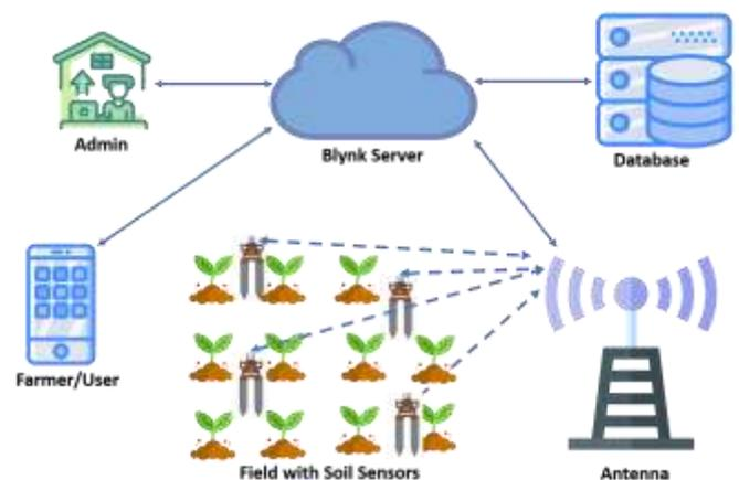
Fig 3.1 system architecture
