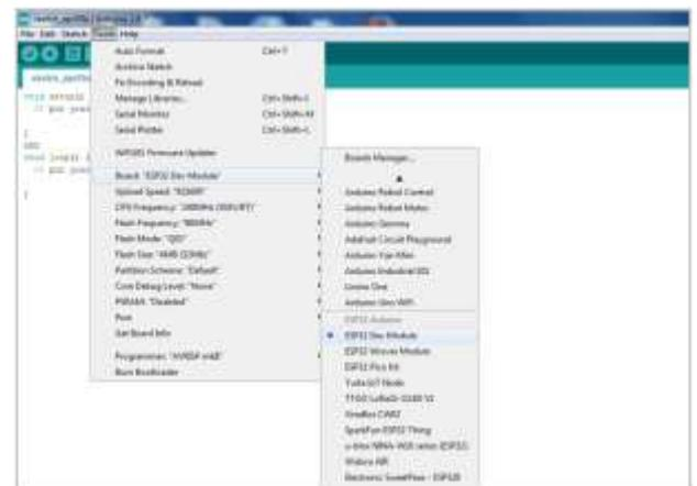
Figure 4.3 Selecting ESP32 on sketch\_apr
