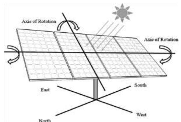
Figure 1 – Representation of a Solar Tracker
