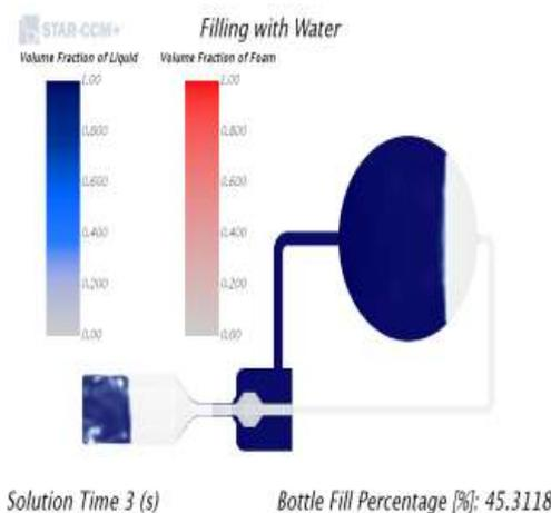
Fig: 4.1 foam factor and volume factor after 3 sec
