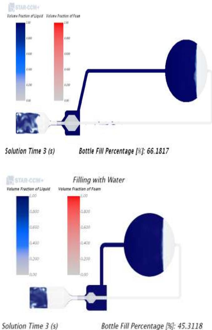
Fig: 4.5 Bottle fill percentage at optimum design
