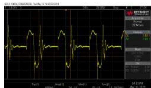
Fig.6: Output of Transmitting Coil
