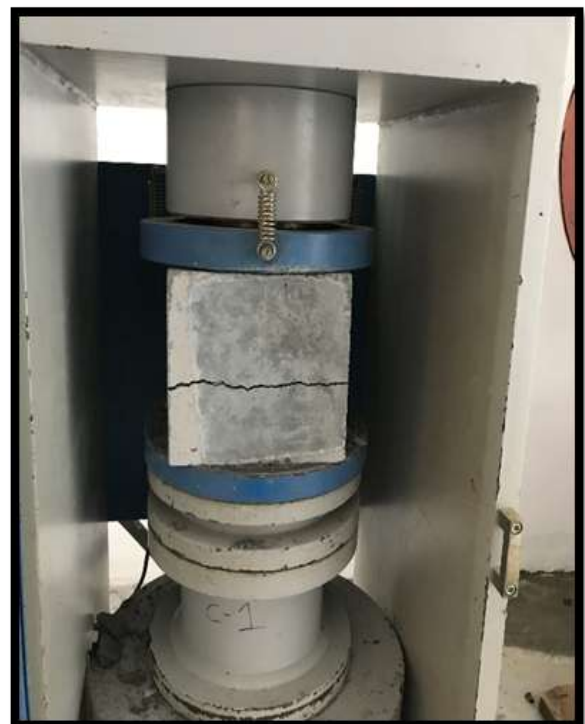
Figure 2. Concrete Member in Compression Testing Machine
