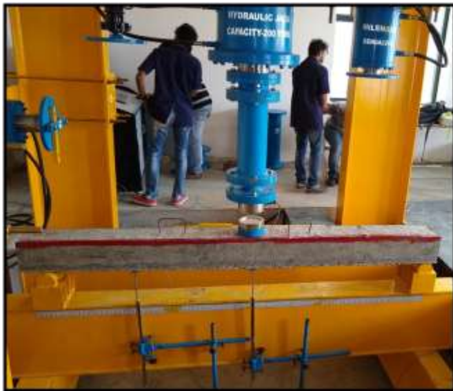
Figure 6. Beam on Loading Frame
