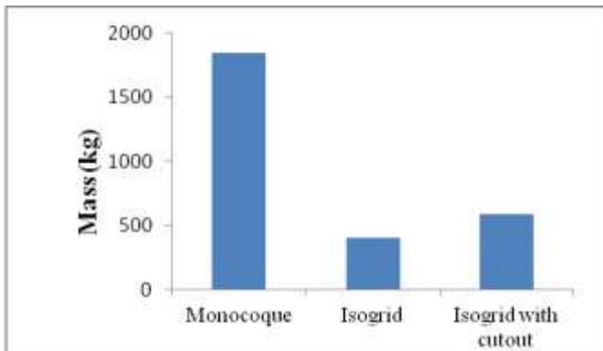
Fig 7. Comparison of mass of structure for monocoque, isogrid and isogrid structure with cutout
