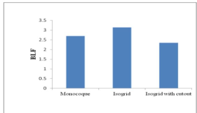
Fig 6. Comparison of Buckling load factor for monocoque, isogrid and isogrid structure with cutout
