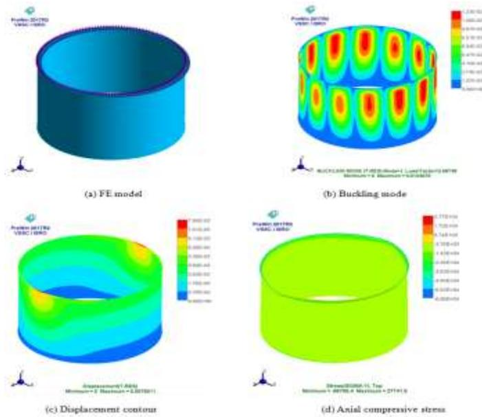
Fig 3. Monocoque Structure
