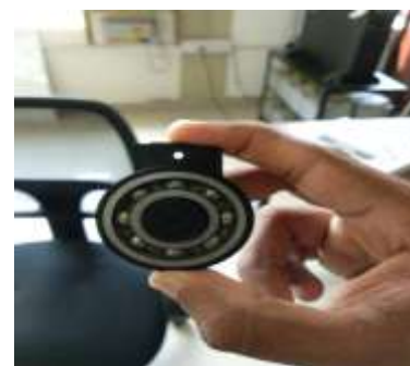
Fig - 6: 3D printed bearing clamp and shaft
