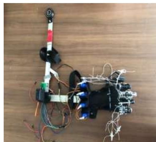
Fig -12: Final prototype of hand exoskeleton
