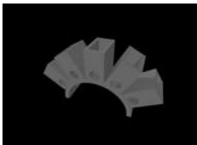
Fig - 4: Design of structure to hold servomotor
