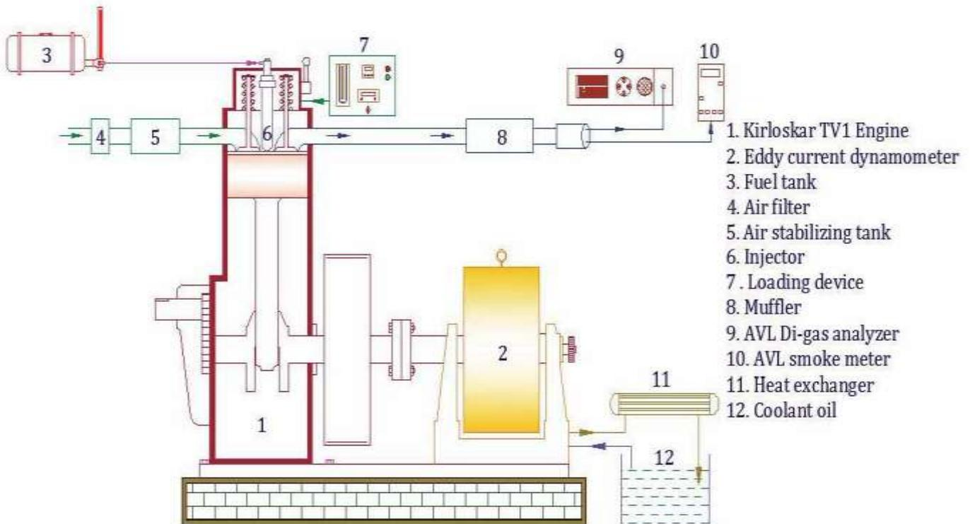
Fig. 2 Experimental setup (Kirloskar TV-1 Engine)
