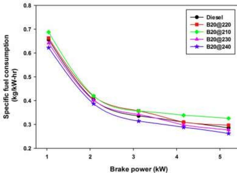
Fig. 4 Variations of specific fuel consumption with brake power
