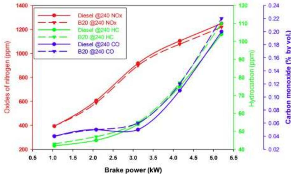
Fig. 9 Comparison of CO, HC and NOx emission
