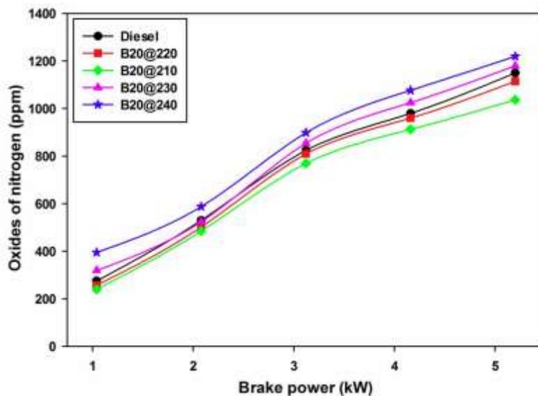
Fig. 6 Variations of NO<sub>x</sub> emission with brake power
