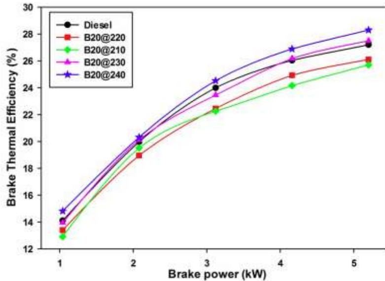
Fig. 3 Variations of brake thermal efficiency with brake power
